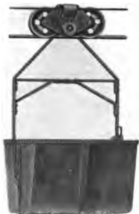
Fig. 9. TRAMWAY CAR, With Bleichert Patent Automatic Overhead Grip.
