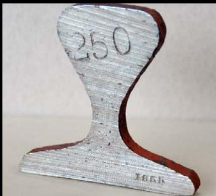
Figure 4: T-Rail Section, Nassau Hall, 1855. The South Trenton Iron Company rolled the first American T-rails with this 3 ½ in.-tall profile, sometimes called a "pear" rail, in 1846. After a fire destroyed much of Nassau Hall at Princeton University in 1855, architect John Notman used Trenton Iron Company T-rails as floor beams in the reconstruction. Seeley Mudd Library, Princeton University. C.W. Zink, 2013
